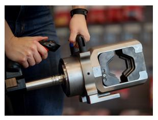
DV350 is a powerful and efficient crimp head with 35 tons crimp force. The head is used together with the electrically driven pump PS710 (the battery powered version, PS710E, is also available) or foot pump P4000, which makes the DV350 exellent for both mobile and stationary work.
