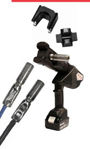
Unique system for aluminium crimping in the 1300 system. The system is designed for low voltage applications (1 kV) and is adapted for ground-covered cable. The number of punches and matrixes has decreased from the previous 21x (including prerounding) to 3 punches and 3 matrixes for the indent crimping of both round and sector-shaped Al conductors in the range 50-240 mm².
