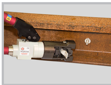
Crimp the Elpress cable clip using the appropriate tool.
