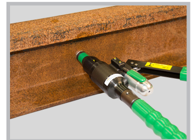
Turn the assembly tool onto its front section. Squeeze the handle until you hear a "click". Railbond will be firmly attached once you have tightened the joint with the torque wrench.
