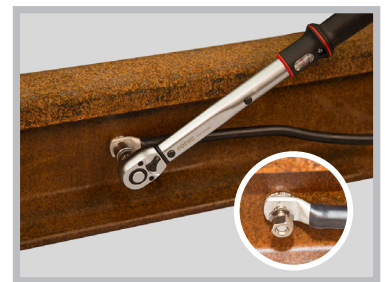
Place the cable clip on the bolt. Always use the supplied washer and nut and also the torque wrench according to recommendations.
